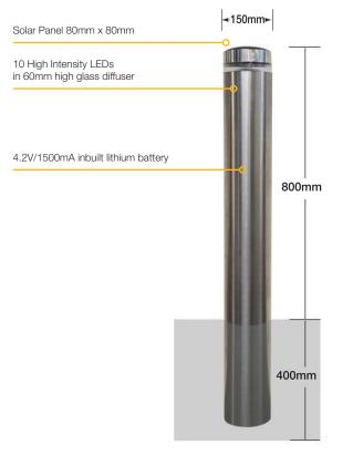
Suitable for inground or bolt-down installation
